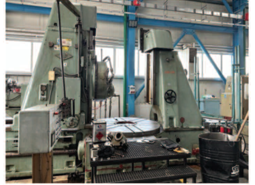
Diameter 3000mm 30 Module Gear Milling Cutter
