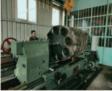
Diameter 1500 Length 6000mm Universal Lathe
