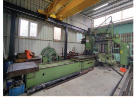
1300x1300x5000mm Gantry Milling
